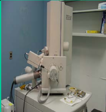
Materials characterization and in-situ mechanical testing with environmental capabilities
